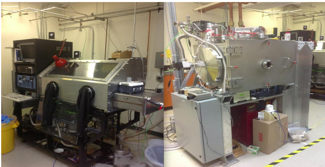
Fig. 1: Evaporator 1 (left) and Evaporator 2 (right)
